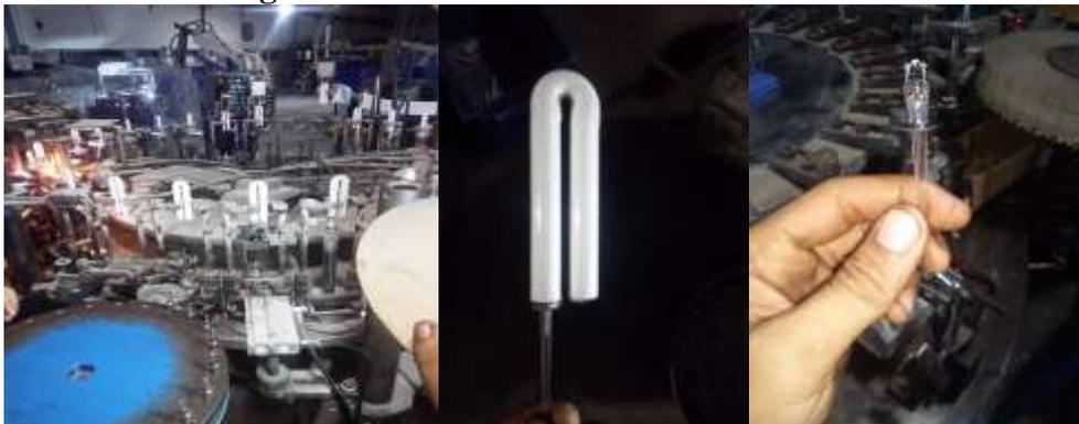
Gambar 5. Proses Mesin Pasang Filamen
