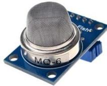
**Gambar 2. Tampilan Sensor Gas MQ-6**
